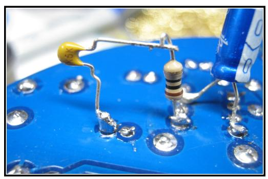
10 ohm resistor soldered on pin 5 and the .1uf cap attached to the left side of the 10uf cap ...where the grounding rays are.
