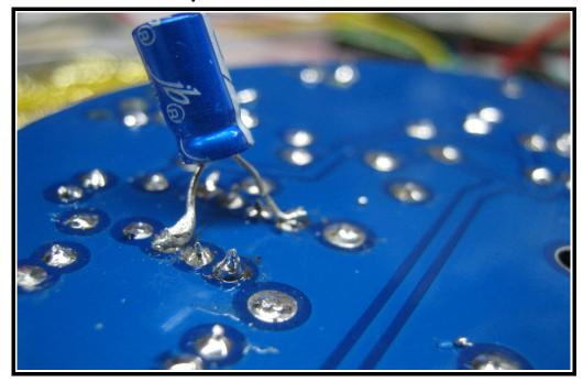
When viewed upside down pin1 on the 8pin device is upper right and has a square pad so solder 10uf + on pin7 and - to pin4
